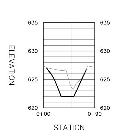
3 CROSS SECTION C-C' PROPOSED GROUND ELEVATION
